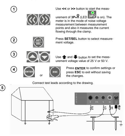
Connect the current electrode driven into ground to the **H** socket of the meter, Connect the voltage electrode driven into ground to the **S** socket of the meter, Connect the tested earth electrode to the **E** socket of the meter,
