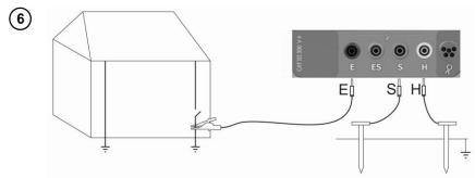
Connect the current electrode driven into ground to the **H** socket of the meter, Connect the voltage electrode driven into ground to the **S** socket of the meter, Connect the tested earth electrode to the **E** socket of the meter.
