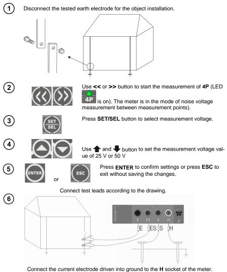
Connect the voltage electrode driven into ground to the S socket of the meter.
