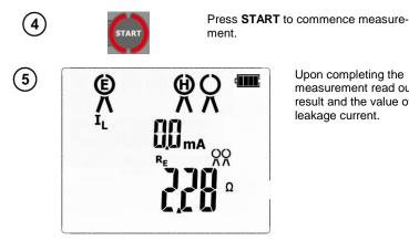
Upon completing the measurement read out the result and the value of the leakage current.
