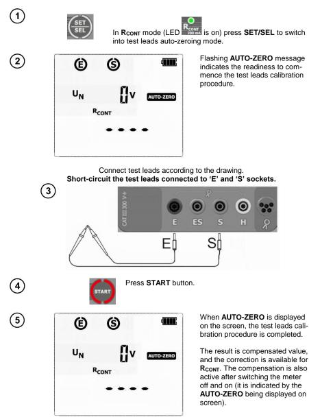
In order to delete compensation (restore default calibration) proceed with the above steps with open (not shorted) test leads. In the place where the result is expected **oFF** message will appear (test leads compensation is now deactivated ). When the procedure is completed **AUTO-ZERO** message will disappear from the screen.
