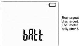
Rechargeable batteries completely discharged. The meter switches off automatically after 5 seconds.
